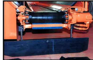
ROLLER CHAIN DRIVEN, HEAT AND OIL RESISTANT CONVEYOR With FLEXIBLE ROAD EDGE MATERIAL STOP
