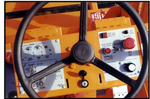
Movable CONTROL STATION includes all machine functions and positions for all options.
